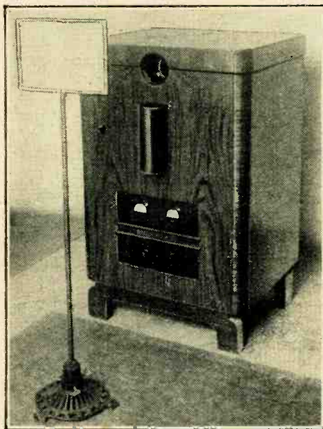
The Mihaly television receiver shown at the recent Radio Exhibition in Berlin. This system employs a stationary mirror drum, with a rotating reflecting mirror, and an external screen on which the picture is projected. The system was described in the issue of The Wireless World of September 15th, 1933.
